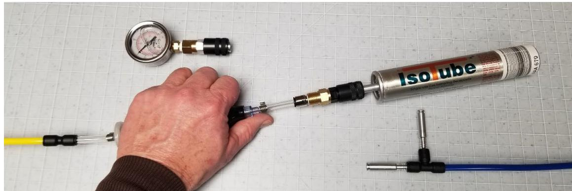
6. Disconnect the IsoTube and re-connect the sample inlet port to the chuck.
